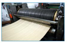
LECTROFLUOR coating prevents food particles from sticking to doughformer rollers. Permits cleanup without caustics.
