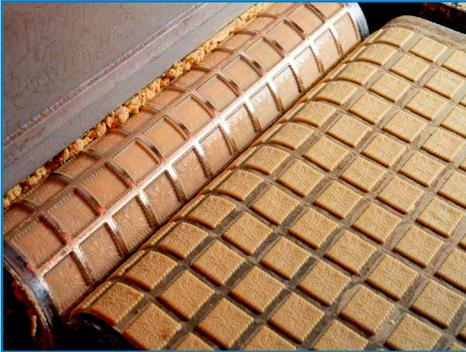
*A cookie manufacturer eliminates frequent production downtime to change batter-clogged cookie molds and also reduces mold replacement by treating the molds with an FDA/USDA-compliant NEDOX coating. Other food processors solve mold release, cleanup and sanitation problems by specifying NEDOX for molds, extrusion pistons and dies, filling nozzles, rollers, trays, kettles and blades.*
